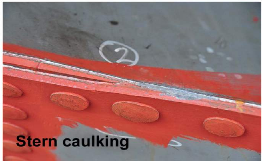
Fig 9 Caulking Rivet Joint Lap Joint.
